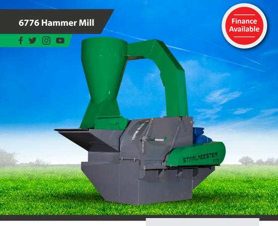
The 6776 is designed to handle ANY type of material, any grain type, maize on the cob, maize stalks, and any grass type. It is designed to handle the very popular B70 round bales and also whole square bales without having to take it apart.
