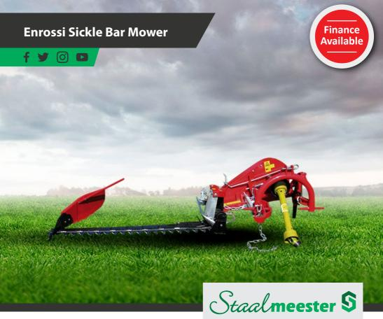
Ideal for small farms. Built to adapt to any type of land. The double action cutter bar ensures a sharp clean cut on any type of grass. The safety breakaway bar helps protect the cutter from obstructions in the field.
