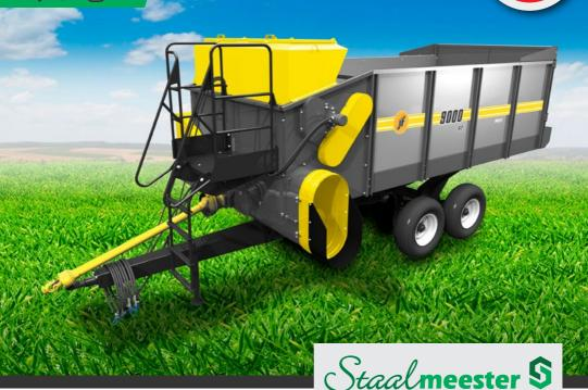
The sidewalls are galvanized and this results in more strength with less weight. JF Taurus 9m³ Forage Wagon was developed to be the ultimate option for the producer when harvesting. Its technological features meet all producers' needs, combining high productivity with low maintenance costs.
